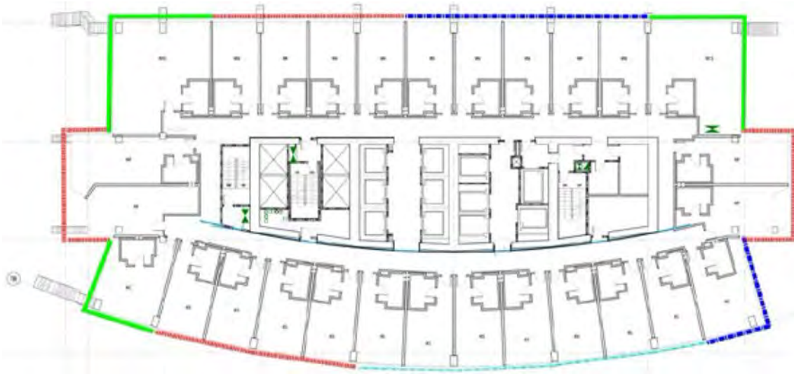
Figure 2. Typical hotel floor plan showing rooms arranged around a narrow core. Courtesy AC Martin.
